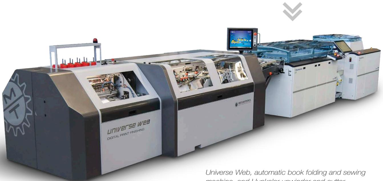
*Universe Web, automatic book folding and sewing machine, and Hunkeler unwinder and cutter.*
